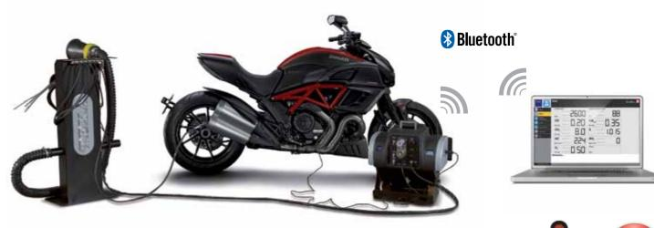
TTC is a universal device for checking correct belt tension. It can be used on all belt types and all vehicle types and measures using a sensitive microphone that analyses resonance frequency after the belt has been tightened. It is entirely wireless and self-powered with rechargeable batteries. It requires no additional tools as it displays the test results directly on its graphic display, emitting a beep once measurement is complete.
