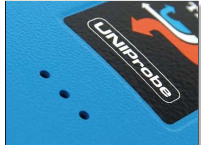
Operating status LEDs
