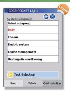
The software's self-diagnostic resources allow you to choose which electronic system you wish to work on by prompting you with a simple, intuitive list of systems the vehicle is equipped with.
