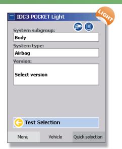
Once you have selected the system family, select the specific system and version of the vehicle you are working on. AXONE Smart now presents you with a list of available self-diagnostic tests.
