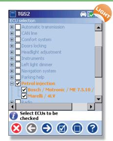
Thanks to the TGS2 function, AXONE Smart lets you analyse all the vehicle's control units automatically, without having to diagnose them one by one.
