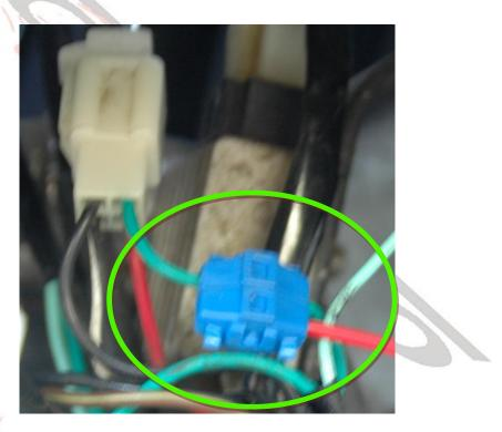
Next you must cut the black/red wire of the connector of the ignition unit. Make sure you can still connect a wire to it. Using the attachment supplied in this kit, you must connect the new red wire (coming from the ignition lock) to the black/red wire. Connect it to the side that is still in the connector of the ignition unit. You can now attach the new ignition unit to the quad.
